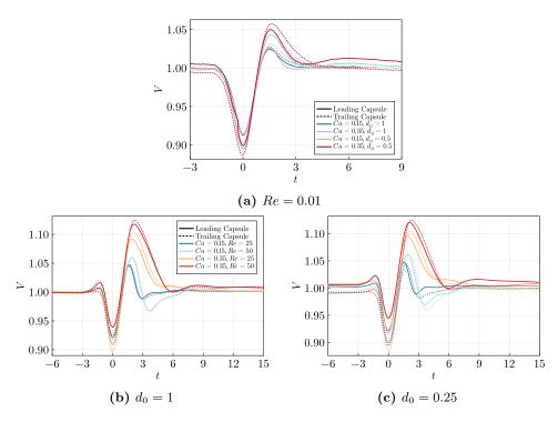
**Figure 5.15:** Temporal evolution of V of the leading and trailing capsules at different Ca, Re and  $d_0$ .
