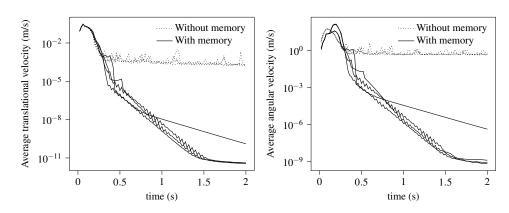
Figure 2.6: Time evolution of the average velocity for a system of 750 spheres settling in a box. Dotted line: no memory term in the contact model. Solid line: memory term in the contact model.
