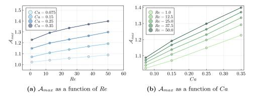
**Figure 5.8:** Maximum area  $\mathcal{A}_{max}$  as a function of Re and Ca for a single capsule passing through the corner.
