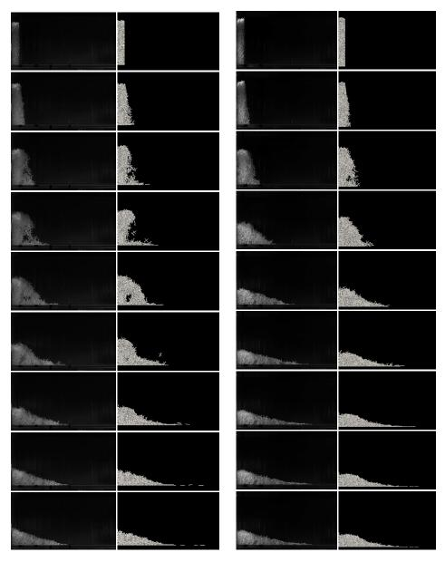
Figure 3.3: Snapshots of a top-driven collapse with an initial aspect ratio  $H_0/L_0 = 6$ . Left: experiments. Right: simulation. Time increment between each frame: 0.145s. Videos of this collapse are available online at https://youtu.be/yzlzn\_XrkJA.
