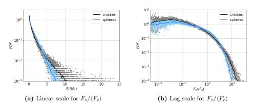
Figure 3.12: Probability density function (PDF) of the contact force magnitude  $F_c$  divided by the average contact force magnitude  $\langle F_c \rangle$  just before the gate is opened, in the cases of assemblies of crosses (black) and spheres (blue).
