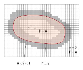
Figure 6.1: Schematic of the Eulerian description of a capsule: the red line denotes the location of the membrane, located in cells where 0 < c < 1; while the shaded area denotes the location of the membrane neighborhood corresponding to  $\tilde{\Gamma} = 1$ .
