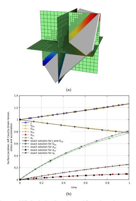
**Figure 6.8:** (a) Surface Jacobian J around a rotated flat membrane subject to a strech increasing linearly along the membrane. The membrane is represented in grey. (b) Corresponding strains, stresses and elastic acceleration and comparison with their analytical solutions, sampled at x = 0.25.
