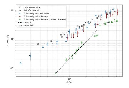
**Figure B.1:** Non-dimensional final x-displacement of the center of mass of the granular assembly (diamond symbols) and non-dimensional run-out distance (all other symbols) as a function of the initial aspect ratio.
