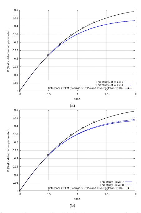
**Figure 6.10:** Convergence analysis of the fully Eulerien method in space (a) and time (b) for the case of an initially spherical neo-Hookean capsule in a shear flow in three dimensions. The Capillary number is 0.2.
