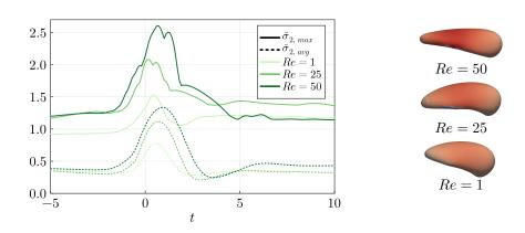
**Figure 5.10:** Left: Maximum and average tensions in the capsule at Ca = 0.35 and Re = 1, 25 and 50. Right: Capsule shape colored by  $\tilde{\sigma}_2$  when  $\tilde{\sigma}_{2, max}$  reaches its maximum.
