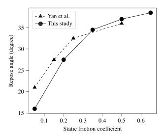
**Figure 2.7:** Variation of the repose angle  $\theta$  with the static friction coefficient  $\mu_c$ . Solid line: this study. Dashed line: adapted from Yan et al. [211]
