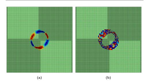
**Figure C.3:** Visualization of the body force term in the x-direction (left) and the IBM stencils defined by a noisy field (right) in the case of a two-dimensional capsule in a shear flow where a forced gird refinement is imposed in parts of the computational domain.
