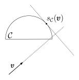
**Figure A.2:** An example of a support mapping  $s_{\mathcal{C}}(v)$  for the convex  $\mathcal{C}$  in the direction v.
