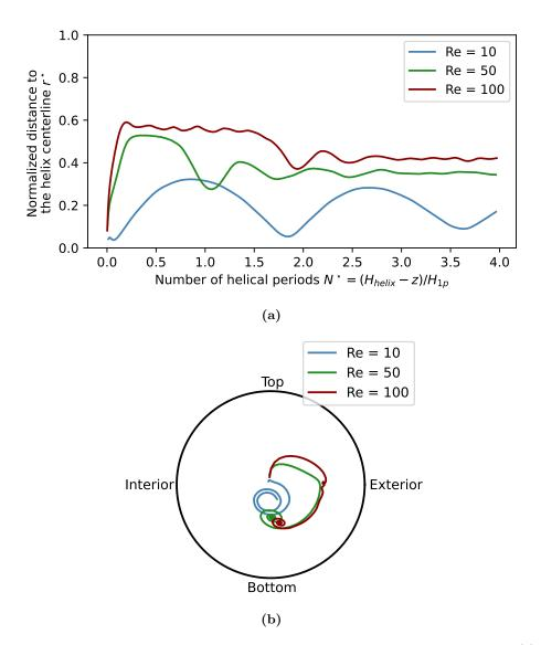
Figure 4.18: Trajectory of a solitary capsule in the helix at Re = 10, 50, 100: (a) normalized distance from the helix centerline; (b) radial migration in a plane orthogonal to the helix centerline.  $N^*$  corresponds to the number of revolutions around the vertical axis of the helix.
