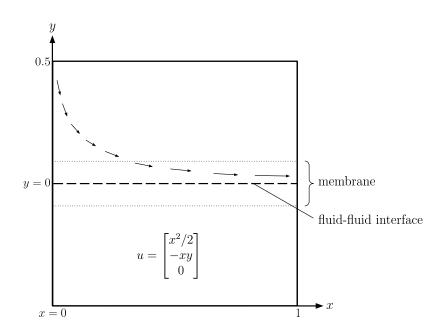
**Figure 6.6:** Elongational flow field leading to membrane stretch varying linearly in the x-direction.
