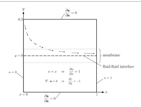
Figure 6.4: Elongational flow field leading to a constant membrane stretch.
