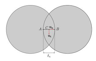
**Figure 2.2:** In soft-body DEM, a contact is modelled with an overlap – Please note that the overlap is intentionally magnified here for visual purposes.
