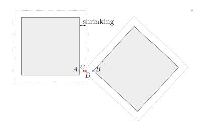
Figure A.5: When two particles are colliding, the access to the contact information is performed by a second call to the GJK algorithm on slightly shrinked versions of the particles. In this schematic (not to scale), the dotted lines represent the original shape of the particles and the solid lines correspond to their shrinked version.
