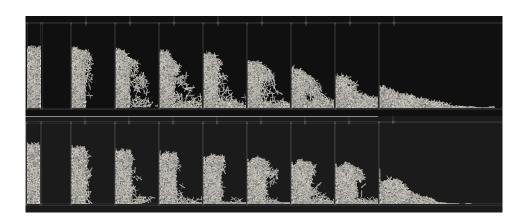
Figure 3.16: Snapshots of simulations with and without memory in the contact model. Top: with memory. Bottom: without memory. The frames are taken at the following times: t = 0s, t = 0.15s, t = 0.30s, t = 0.45s, t = 0.60s, t = 0.75s, t = 0.90s, t = 1.05s and t = 3.00s.
