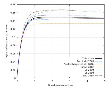
Figure 4.7: Taylor deformation parameter of an isolated capsule undergoing elastic and bending stresses in a shear flow. The capillary number is Ca = 0.05 and the non-dimensional bending coefficient is  $\tilde{E}_b = 0.0375$ .
