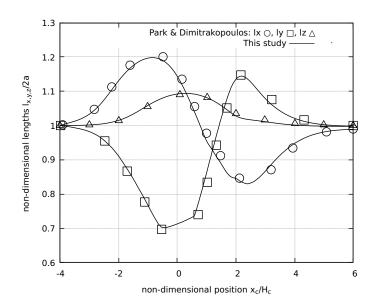
Figure 4.9: Non-dimensional lengths of the capsules in the three directions x, y and z with respect to the non-dimensional x-position of the center of the capsule. Results are compared to [145].
