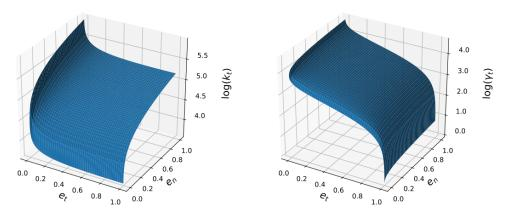
**Figure 3.18:** Surface plots of the tangential parameters  $k_t$  and  $\gamma_t = \frac{\eta_t}{2m}$  for  $e_n$  and  $e_t$  varying from 0 to 1.
