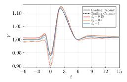
Figure 5.17: Effects of the initial interspacing distance  $d_0$  on the evolution of the capsules velocities V at Ca = 0.35, Re = 50.
