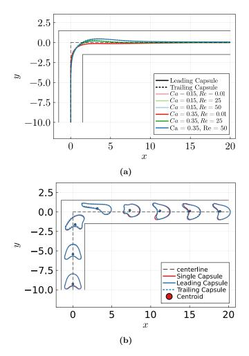
**Figure 5.13:** (a) Trajectory of the two capsules at different Ca and Re. (b) Outlines of the leading and trailing capsules at Ca = 0.35, Re = 50,  $d_0 = 0.25$ , with comparison to a single capsule.
