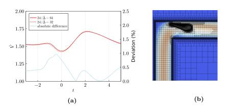
Figure 5.2: (a) Centroid velocity of a capsule at Ca = 0.35 and Re = 50 for two grid resolutions: 32 grid cells per initial diameter (red dotted line) and 64 grid cells per initial diameter (red solid line). The blue curve denotes the deviation in the centroid velocities for these two grid resolutions. (b) Corresponding shape and grid resolutions of the capsule and the flow field: blue means zero velocity and red means large velocity.
