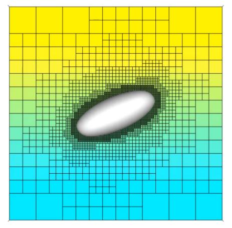
**Figure 6.9:** A neo-Hookean capsule represented by the fully Eulerian method in a shear flow. The color field represents the magnitude of the x-component of the velocity.
