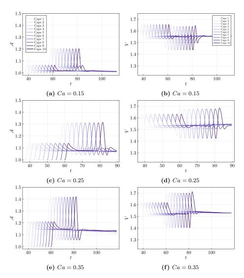
Figure D.2: Time evolution of the reduced areas and velocities of ten capsules at Re = 50 and  $d_0 = 1$  for Ca = 0.15, 0.25 and 0.35.
