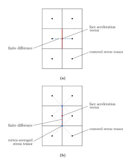
**Figure 6.2:** Numerical scheme to obtain a face-centered differentiation of a cell-centered tensorial quantity. (a) Differentiation along the normal of the considered face (simple finite differencing). (b) Differentiation along a tangential direction to the considered face (involves vertex-averaging before differentiating).
