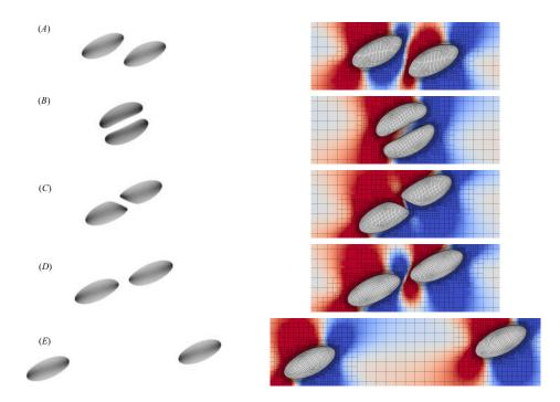
Figure 4.12: Snapshots of the interception of two neo-Hookean capsules in a shear flow. Left: Boundary Integral results of Lac et al. [115]. Right: This study. The color field corresponds to the vertical component of the velocity (rescaled for each snapshot).
