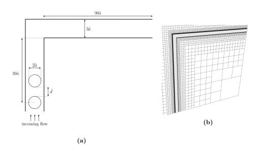
**Figure 5.1:** (a) Schematic of the geometry of the fluid domain. The channel has a square cross-section of side length  $3\tilde{a}$ . (b) Visualization of the full channel and the computational grid over the symmetry plane of the channel.
