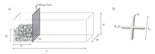
Figure 3.1: Schematics of the experimental setup: (a) the dam break apparatus and (b) the shape of the particles.
