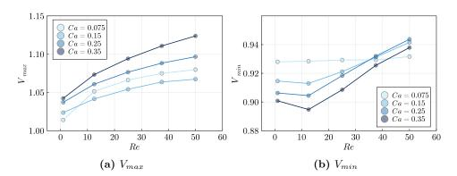
**Figure 5.9:** Maximum (minimum) velocity  $V_{max}$  ( $V_{min}$ ) as a function of Re and Ca for a single capsule passing through the corner.
