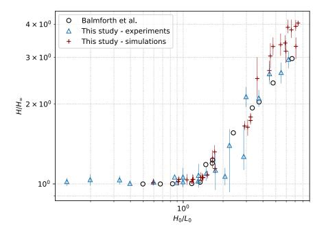
**Figure 3.8:** Non-dimensional height  $H_0/H_\infty$  as a function of the initial aspect ratio  $H_0/L_0$ . Error bars are depicted with vertical segments.
