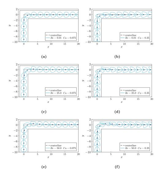
Figure 5.11: Sequence of Capsule outlines for different Ca and Re. The time between each frame is t = 1.5.
