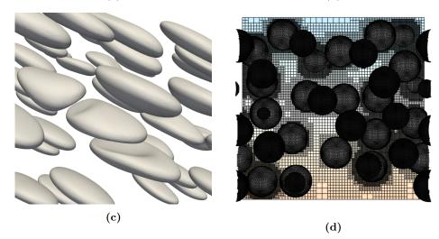
**Figure 7.1:** Qualitative view of sheared suspensions of 100 initially spherical capsules: (a) initial configuration at a volume fraction  $\phi = 5\%$ , (b) configuration at  $\phi = 5\%$  after 5 reference time units, (c) zoom on interacting capsules located in the lower right corner of (b), and (d) vizualization of the adaptive grid at time t = 0 and at  $\phi = 25\%$ . The open capsules are a vizualization artifact due to periodic boundary conditions.
