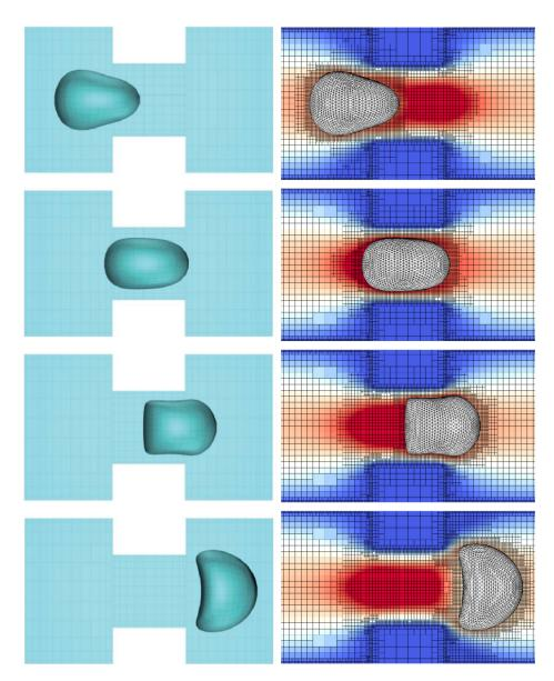
**Figure 4.8:** Snapshots of the capsule as it flows through the constriction. Left: Park & Dimitrakopoulos [145]; Right: this study.
