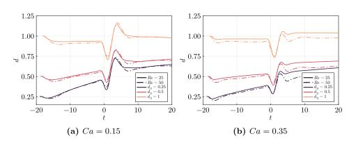
**Figure 5.16:** Temporal evolution of d for different initial interspacing distance  $d_0$  and Reynolds number Re.
