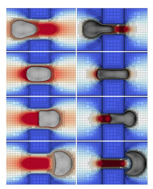
**Figure 4.15:** Qualitative comparison of a capsule flowing through a constricted channel: when the constriction size is equal to the initial diameter of the capsule (left); and when the constriction size is equal to half of the initial diameter of the capsule, with a finest Eulerian grid resolution of 100 cells per initial diameter (right). Color field: *x*-component of the velocity field.
