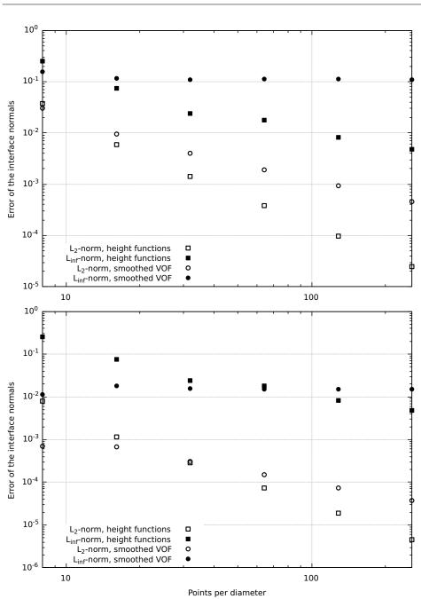
Figure 6.3:  $L_2$ -error and  $L_{\infty}$ -error on the normal vectors for a circular membrane, in the whole membrane region  $\tilde{\Gamma}$  (top) and restricted to the interfacial cells (bottom). Two methods to compute the normal vectors in the interfacial cells are compared: (i) from the normalized gradient of the mollified VOF function, and (ii) from the height functions method presented in [153].
