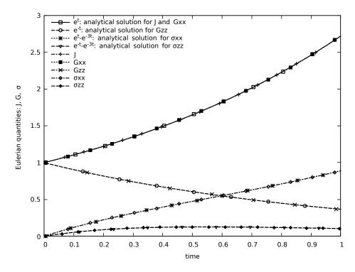
Figure 6.5: Strains and stresses in a flat horizontal membrane located at y = 0 and subject to a constant stretch.
