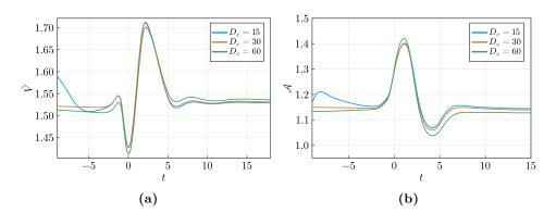
Figure 5.3: Centroid velocity (a) and normalized area (b) of a capsule flowing through a corner from three distinct normalized release distances  $D_c = 15$ , 30 and 60, at Re = 50 and Ca = 0.35.
