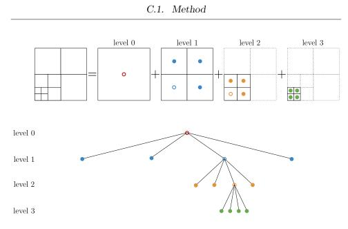
**Figure C.1:** Tree structure of a quadtree grid. The filled circles represent leaf cells while the open circles represent parent cells.
