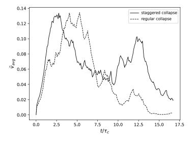
Figure 3.10: Comparison of the average non-dimensional translational particle velocity versus non-dimensional time for a staggered collapse (solid line) and a regular collapse (dashed line) in the case of an initial aspect ratio  $a = H_0/L_0 = 1.75$ . The only difference between the two collapses is the random initial packing.
