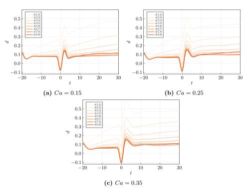
Figure 5.19: Temporal evolution of d for a train of 10 capsules at Re = 50 and  $d_0 = 0.125$  for (a) Ca = 0.15, (b) Ca = 0.25 and (c) Ca = 0.35.
