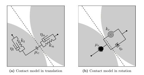
**Figure 2.3:** The linear spring-dashpot contact model as a mechanical analog. The dashed line represents the tangential contact plane.
