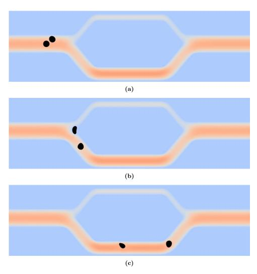
**Figure 7.2:** (a) Initial pre-collision configuration. (b) Collision of the top capsule with the channel walls. (c) Post-collision configuration.
