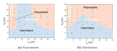
Figure 3.6: Flow maps from (a) experiments and (b) simulations. Each cross represents an experiment or a simulation. Two flow regimes are identified: repeatable and intermittent; and two collapse behaviors are reported: top-driven (observed in all configurations) and buckling (observed only for narrow columns).
