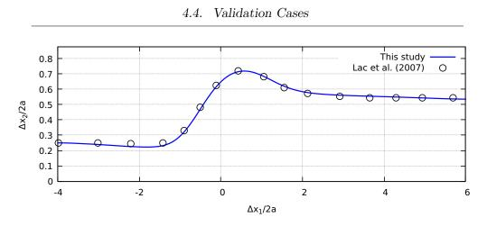
Figure 4.13: Non-dimensional vertical gap  $\Delta x_2/2a$  against the non-dimension horizontal gap  $\Delta x_1/2a$  between the centers of the two capsules. The results from this study are compared to Lac et al. [115].
