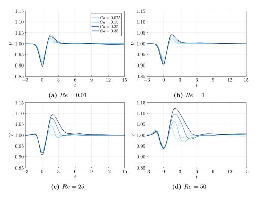
**Figure 5.4:** Temporal evolution of the capsule centroid velocity V at fixed Reynolds numbers.
