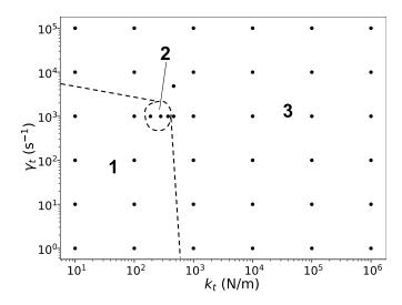
**Figure 3.17:** Variation of the flow behavior with respect to the tangential parameters. Each dot corresponds to a simulation with specific tangential parameters  $(k_t, \gamma_t)$ . Region 2 correctly reproduces experiments. Region 1 leads to avalanches that collapse like convex particles, i.e., the base of the pile drives the motion. Region 3 leads to fully entangled systems that do not collapse.
