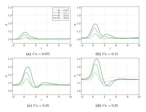
Figure 5.7: Temporal evolution of the capsule surface area  $\mathcal{A}$  at fixed Capillary numbers.
