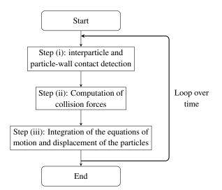
Figure 2.1: Top-level view of a soft-body DEM algorithm
