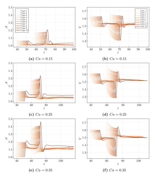
Figure 5.18: Time evolution of the reduced areas and velocities of ten capsules at Re = 50 and  $d_0 = 1/8$  for Ca = 0.15, 0.25 and 0.35.
