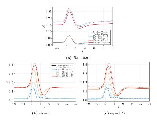
**Figure D.1:** Temporal evolution of the reduced area  $\mathcal{A}$  of the leading and the trailing capsules at various interspacings  $d_0$  and various Capillary and Reynolds numbers Ca and Re.
