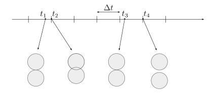
Figure 2.4: Illustration of the error stemming from the latency in the detection of the beginning and the end of the contact. Adapted from Kruggel-Emden et al. [112].
