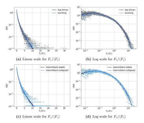
**Figure B.3:** Probability density functions (PDFs) of the contact forces  $F_c$  just before the gate is opened, in the cases of (a-b) top-driven regime (black) with buckling regime (blue); and (c-d) intermittent regime leading to stable (black) and collapsed (blue) behaviours.
