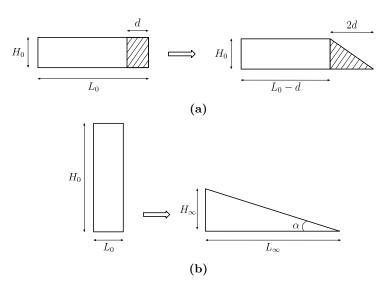
**Figure B.2:** Schematics of the avalanche profiles of the granular assembly for low (a) and high (b) aspect ratios, under the assumption that the slope of the avalanched profile is constant for a given aspect ratio.
