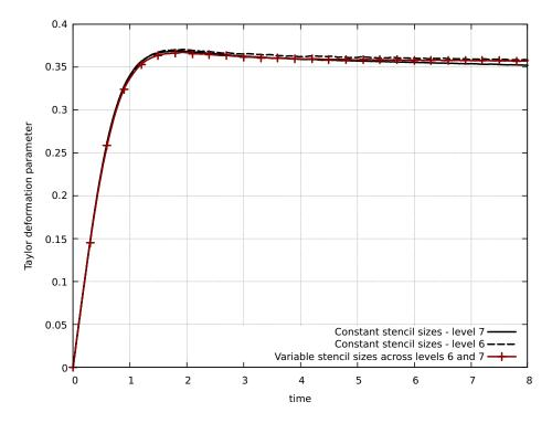
**Figure C.4:** Taylor deformation parameter of a two-dimensional capsule in a shear flow where a forced grid refinement is imposed in parts of the computational domain. Three cases are considered: (i) the membrane is at a constant fine level of refinement (solid black line), (ii) the membrane is at a constant coarse level of refinement (dashed black line), (iii) the membrane spans two levels of refinement (red line).
