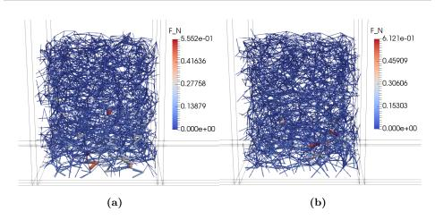
Figure 3.15: Visualization of the force network of two intermittent simulations. Each segment links a contact point to the center of mass of a particle, and is colored according to the magnitude of the normal component of the contact force. (a) The opening of the right gate leads to a granular collapse. (b) The opening of the right gate leads to a stable assembly.
