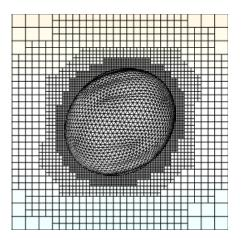
Figure 4.6: A zoomed in snapshot of a buckling membrane at Ca = 0.0125 with a Lagrangian discretization comprising 5120 triangles. This behavior is arising due to the absence of bending stresses, and the buckling wavelength is dependent on the Lagrangian discretization. The color field represents the x-component of the velocity.
