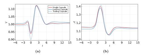
**Figure 5.14:** Temporal evolution of the velocity V and the area  $\mathcal{A}$  of capsules at Ca = 0.35, Re = 50 with  $d_0 = 0.25$ : a comparison of the leading, trailing and a single capsule.
