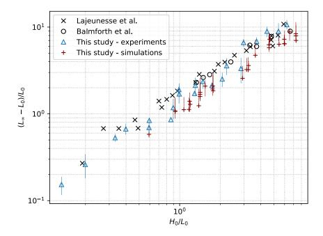
**Figure 3.7:** Non-dimensional runout distance  $(L_{\infty} - L_0)/L_0$  as a function of the initial aspect ratio  $H_0/L_0$ . Error bars are depicted with vertical segments.
