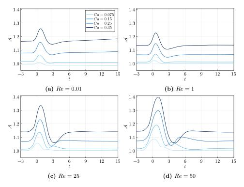
Figure 5.6: Temporal evolution of the capsule surface area  $\mathcal{A}$  at fixed Reynolds numbers.
