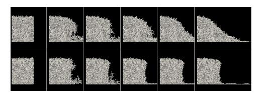
Figure 3.5: Snapshots of a simulated collapsing assembly (top) and of a simulated stable assembly (bottom). The initial dimensions of both assemblies are identical: only the initial microstructure differs between these two intermittent cases. The frames are taken at the following times: t = 0s, t = 0.30s, t = 0.60s, t = 0.90s, t = 1.20s and t = 2.00s.
