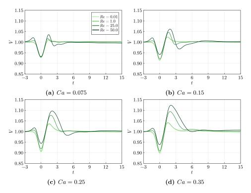
Figure 5.5: Temporal evolution of the capsule centroid velocity V at fixed Capillary numbers.
