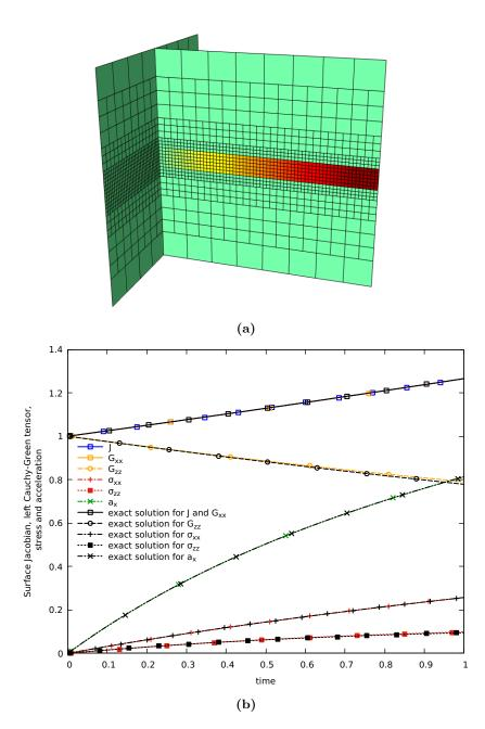
**Figure 6.7:** (a) Surface Jacobien J around a horizontal flat membrane (not shown) subject increasing linearly along the x-direction. (b) Corresponding strains, stresses and elastic acceleration and comparison with their analytical solutions, sampled at x = 0.25
