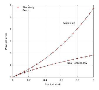
Figure 4.2: Stress-strain response of an isolated flat membrane for the neo-Hookean and Skalak elastic laws. The results from this study are compared to exact expressions derived in [20].
