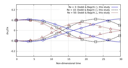
**Figure 4.14:** Non-dimensional vertical gap  $\Delta x_2/2a$  against the non-dimensional time  $\dot{\gamma}t$  for Reynolds number of 3, 10 and 50. The results of this study are compared to Doddi & Bagchi [44].
