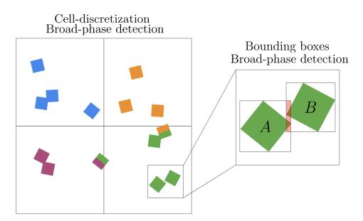
Figure A.1: Two stages of broad-phase detection: space-discretization in cells and bounding boxes. Particles with the same color will undergo the bounding boxes broad-phase detection, and particles which bounded-boxes overlap will launch narrow-phase detection.
