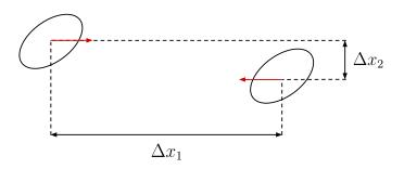
**Figure 4.11:** Schematic of the two capsules in in the shear flow, prior to the interception. The horizontal and vertical gaps  $\Delta x_1$  and  $\Delta x_2$  are defined, and the red arrows represent the velocities of the centers of the capsules.
