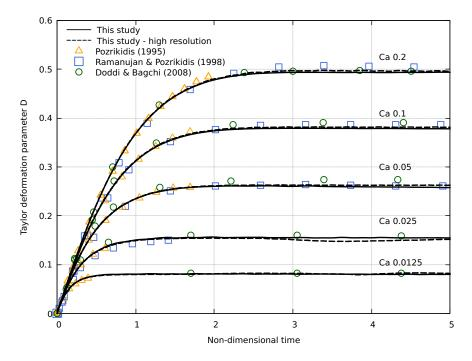
Figure 4.5: Taylor deformation parameter as a function of the non-dimensional time of an initially spherical Neo-Hookean capsule in an unbounded shear flow. The solid line corresponds to 32 Eulerian cells per initial diameter and a Lagrangian discretization using 1280 triangles, while the dashed line corresponds to 64 Eulerian cells per initial diameter and a Lagrangian discretization using 5120 triangles.
