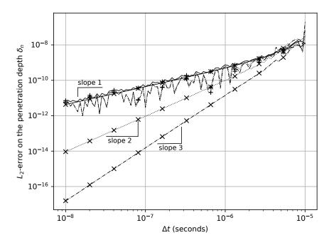
Figure 2.5: Error on the penetration depth  $\delta_n$  of a sphere bouncing on a horizontal plane for the first order Forward Euler scheme (solid line), the second-order Adams-Bashforth scheme (dotted line) and the third order Adams-Bashforth scheme (dash-dotted line). For each scheme, the bouncing sphere is either (i) already in contact with the horizontal plane at t = 0 ("x" markers), or (ii) away from the horizontal plane at t = 0 ("+" markers).
