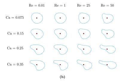
**Figure 5.12:** Outlines of a single capsule passing a corner with (a) maximal area  $\mathcal{A}$  and (b) maximal velocity  $v_{max}$  at various Re and Ca.
